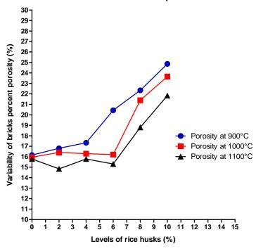
Figure 12. Influence of adjuvant and firing temperature on porometric properties of fired clay bricks
