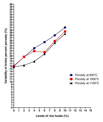
Figure 11. Influence of adjuvant and firing temperature on porometric properties of fired clay bricks
