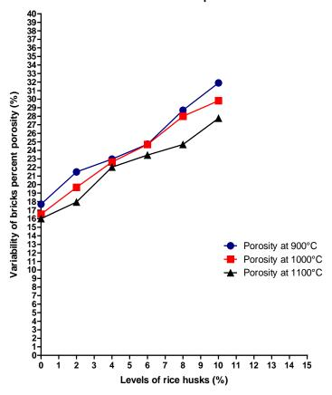
Figure 14. Influence of adjuvant and firing temperature on porometric properties of fired clay bricks
