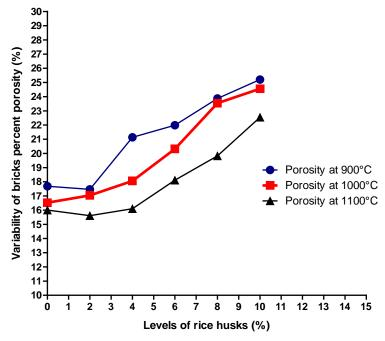
$\textbf{Figure 15.} \ \textbf{Influence of adjuvant and firing temperature on porometric properties of fired clay bricks}$
