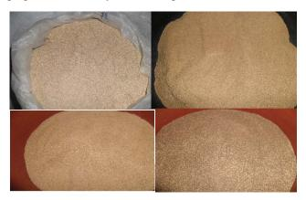
**Figure 6.** Respective particle size cutoff Rice Balls 1000-500 $\mu$ m (photo above left), from 500 to 315 $\mu$ m (photo above right), of 315-125 $\mu$ m (photo below left), and finally the mixture over rice balls clay (photo below right)
