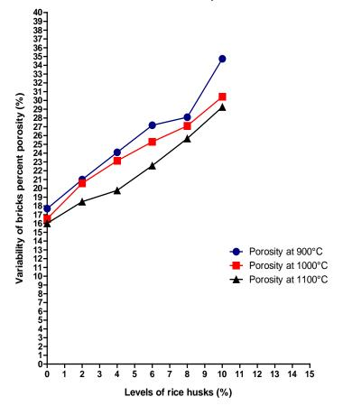
Figure 13. Influence of adjuvant and firing temperature on porometric properties of fired clay bricks
