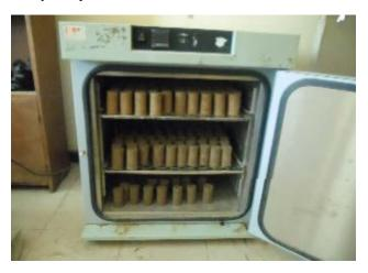
Figure 9. Specimens of bricks in an oven set at a temperature of 105°C
