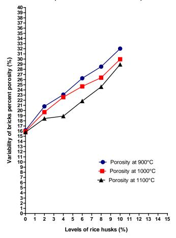
Figure 10. Influence of adjuvant and firing temperature on porometric properties of fired clay bricks
