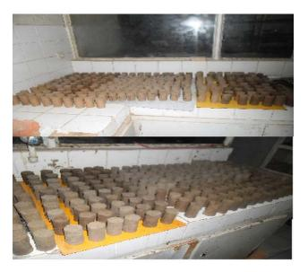
Figure 8. Respective specimens of Badjengo (picture above) and Kalge (photo below) in curing period
